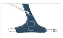
Pass the USB-C cable through the holster, from back to the front.
