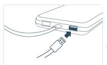
Take the USB/USB-C cable and connect the USB connector to the hub battery.
