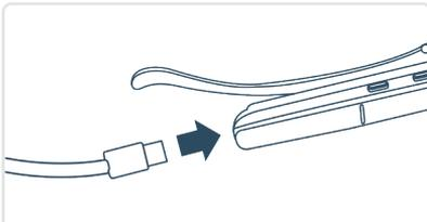
Connect the USB-C cable to the Vuzix M400.
