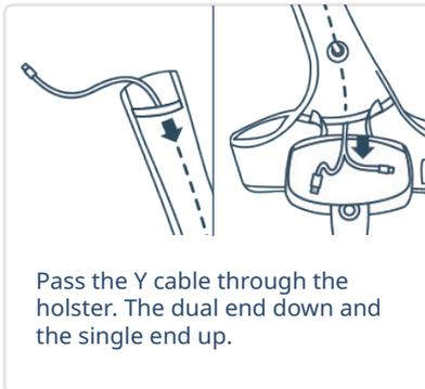
Pass the Y cable through the holster. The dual end down and the single end up.
