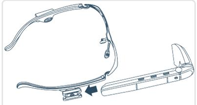
Slide the Vuzix M400 into the frame bracket.
