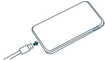
Connect the USB-A port (dual end) to the power bank.
