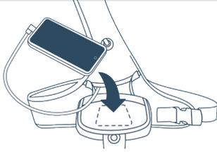
Attach the device to the holster pocket.
