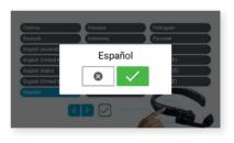
To change the language directly on the device, press and hold the action button  $\rightarrow$ , release it when the desired language is highlighted and go back to XpertEye.
