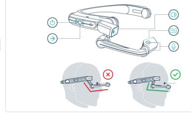
Turn on the HMT device by pressing the power button  $\circlearrowleft$  for 3 seconds. When the HMT device starts up, the RealWear logo is displayed and a startup sound will be heard after a few seconds.
