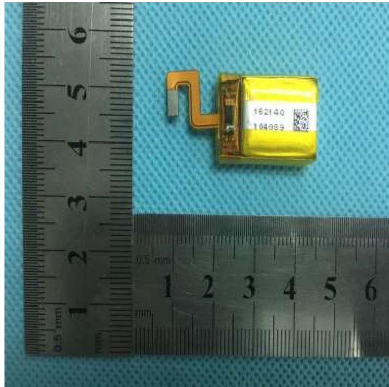
Figure 1 Front view of battery
